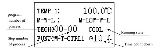
Under the running process mode: press key to view the feeding state, output state, input state, running curve.
