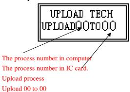
**Upload one by one:** copy the process one by one to IC card.
